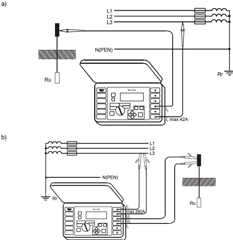
**Fig.22. Method of connecting MZC-310S when measuring the grounding resistance for TN-C, TN-S i TT : a) using two-pole method b) using four-pole method**
