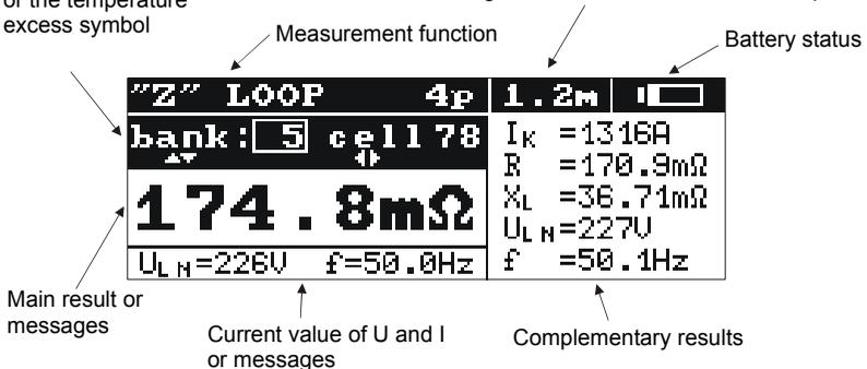
Fig.3. Screen layout in short-circuit loop impedance measurement mode (all results)
