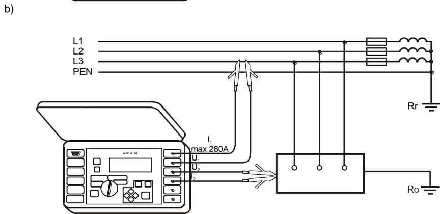
**Fig.17. Verification of the anti-shock protection reliability of appliance's housing using four-pole method for: a) TN networks b) TT networks**
