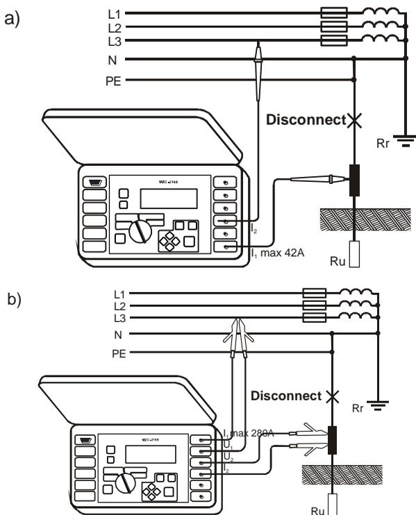
**Fig.23.** MZC-310S connection diagram to be used when measuring the earth resistance for TN-C-S
